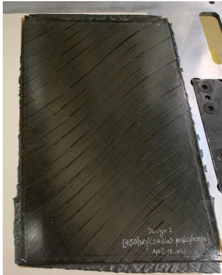
Design 2: highest buckling load compared to the baseline
